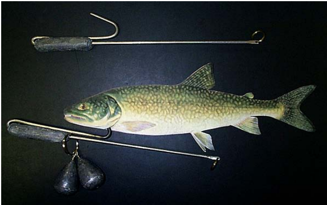
Figure 2: Apparatus used for deep release of lake trout (photo courtesy of D. Reid, Ministry of Natural Resources, Owen Sound)
